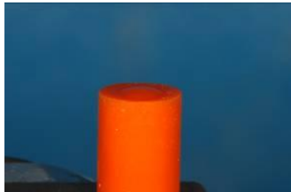
Fig.1 This photo depicts the exceptionally low contact angle of the water bead on the Wash (Light Bodied) material, which shows the hydrophilic properties of Take 1 ® .
