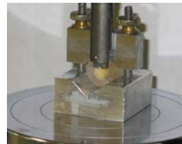
Figure 2: Shear Bond Test Set-Up
